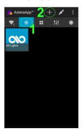
On the AsteraApp<sup>TM</sup> main screen, first press the Targets button (1) and then the "+" sign (2) to add a new target.
